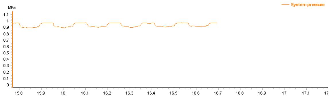
**Incident:** Leaking inlet check valve.
