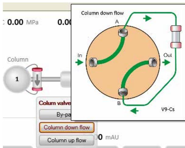
*Result:* The Column valve switches to position **1**.
