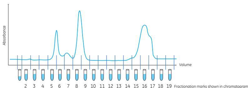
When fixed volume fractionation is used the delay volume is collected at the beginning of fractionation. Fraction collector F9-R saves the delay volume in the first fraction (fraction 1), see the example illustration above. Delay volumes are not indicated with a numerical fraction mark on the chromatogram. Fraction collector F9-C does not save the delay volume as a fraction, instead the delay volume is disposed of in the waste funnel.
