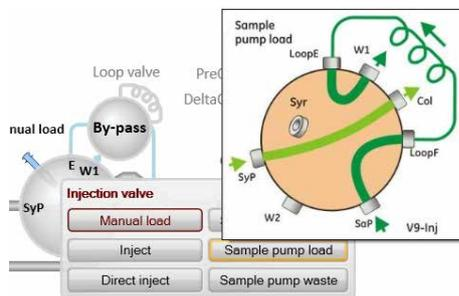
**Result:** The Injection valve switches to **Sample pump load** position.
