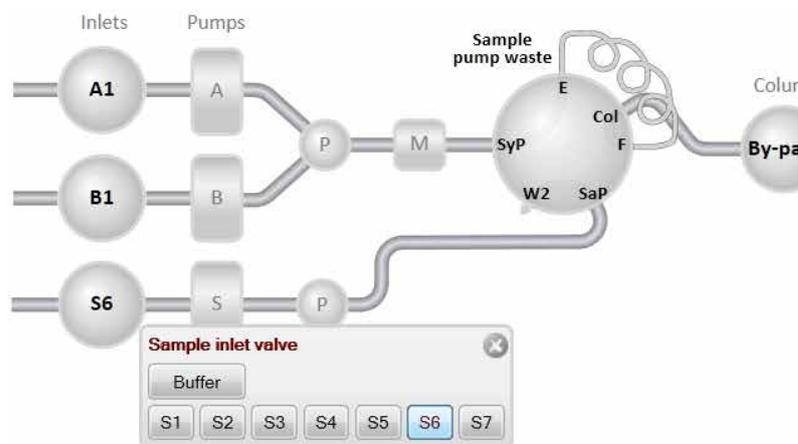
*Result:* the sample inlet valve switches to the selected port.
