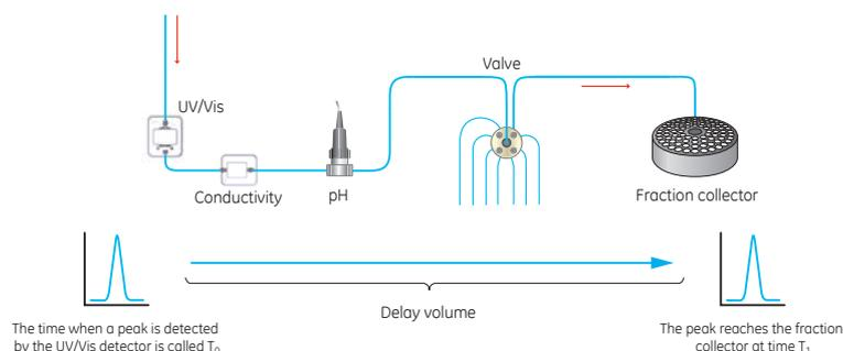
As the delay volume is affected by the length and diameter of the tubing, it should be set according to the tubing and modules used.
