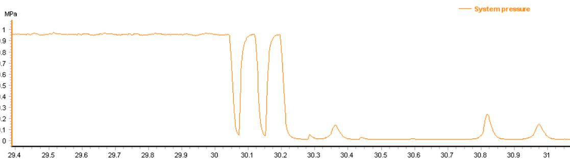
**Incident:** Blocked outlet check valve
