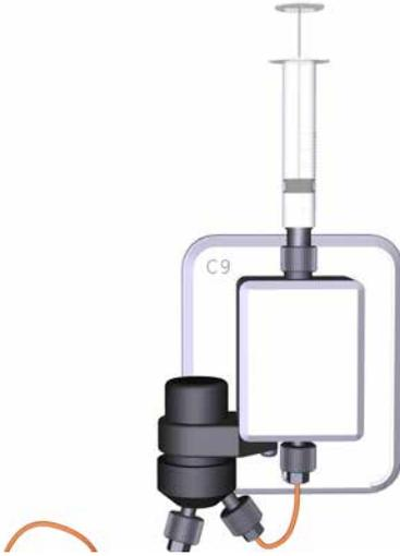
A 3D technical illustration showing a syringe with a clear barrel and a black plunger. The syringe is connected to a rectangular conductivity flow cell labeled 'C9'. The flow cell is mounted on a black base with a motor and various connectors. An orange tube is connected to the bottom of the flow cell. The syringe is inserted into a Luer lock connector on top of the flow cell. |
