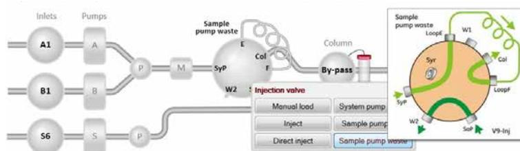
*Result:* The injection valve switches to waste position. This is necessary to achieve a low back pressure during the purge procedure.
