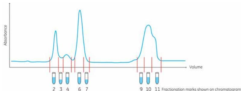
When peak fractionation is used, Fraction collector F9-R collects the delay volumes in the fractions preceding each peak. In the chromatogram above, delay volumes are collected in fractions 1, 5 and 8. The numerical fraction marks for the delay volume fractions are not indicated on the chromatogram. Fraction collector F9-C does not save the delay volumes as fractions, instead the delay volumes are disposed of in the waste funnel.
