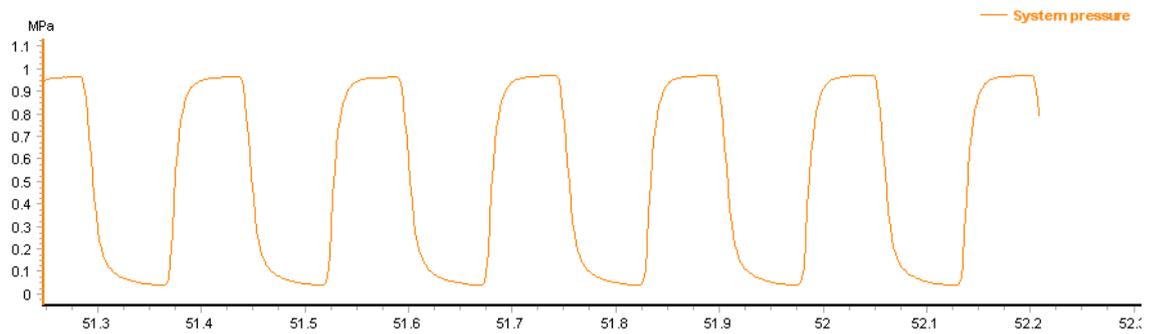
**Incident:** Inlet check valve is loose.
