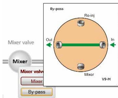
*Result:* The Mixer valve switches to **By-pass** position.
