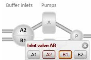
*Result:* The inlet valve switches to the selected port.
