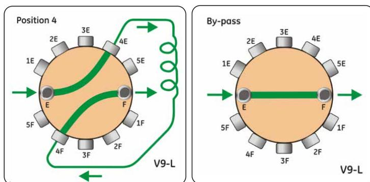
In the **Position 4** example, the loop is connected to loop position 4 and the loop is being emptied.
