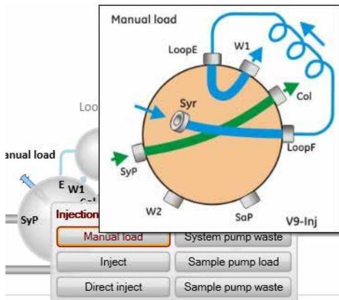
*Result:* Injection valve is set to manual load.
