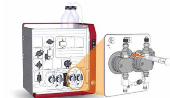
7 Open the purge valve by turning it counter-clockwise about three quarters of a turn. Draw a small volume of liquid slowly into the syringe (with a rate of about 1 ml per second).
