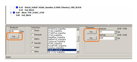
There is one *Var...* button in the *Breakpoint* field and one *Var...* button for each parameter in the *Parameters* field.
