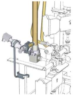
Hollow fibre cartridges are provided with two connections to the permeate compartment, one in each end.
