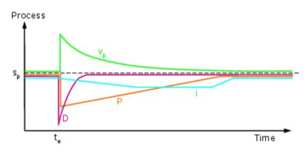
This illustration shows the behaviour of the P, I and D components of a typical PID process control regulator.
