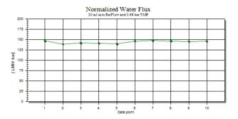
The image shows an example of plotted Normalized Water Flux.
