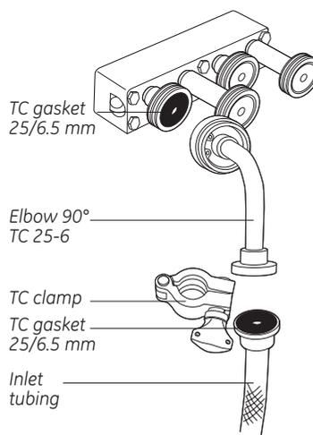
**Connecting air sensor 2 to an inlet tubing**
