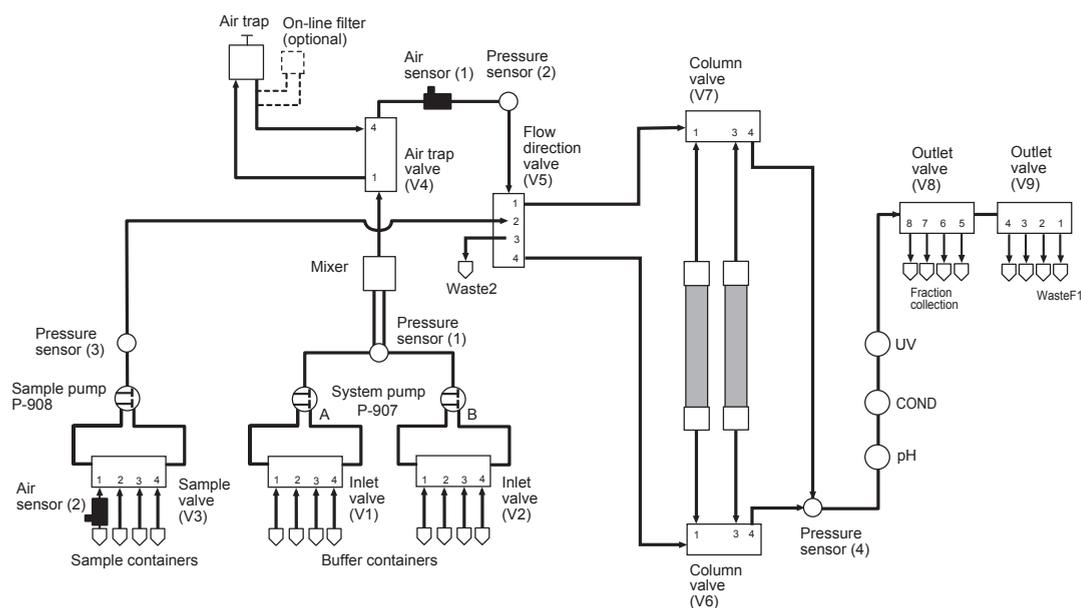
Fig 1-3. The liquid flow path of ÄKTApilot
