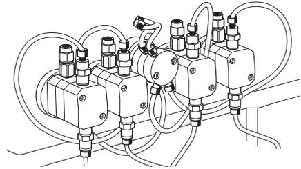
A pressure sensor is connected to pump module A (the left-hand pump heads). The pressure is almost the same in pump module B. The pressure sensor provides an over-pressure alarm function, which is preset in UNICORN.
