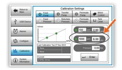
16 Enter the saved **Pf** feed pressure sensor value measured in the gray field marked with *Pressure*.
