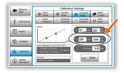
12 Enter the saved **Pp** permeate pressure sensor value in the gray field marked with **Pressure**.
