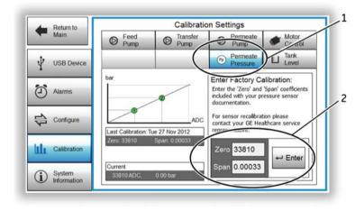
4 Enter the factory settings for the pressure unit connected to the system, in the gray fields (2) marked *Zero* and *Span*.
