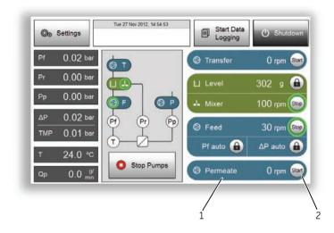
2 Use the displayed keypad to set the desired permeate pump speed (rpm) and tap **OK**.
