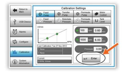
*Result:* The software calculates the correlation between used RPM and achieved flow and the feed pump is calibrated.
