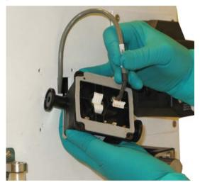
Place the pressure sensor over the fittings for the screws on the chassis so that they match.
