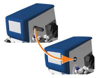
**Note:** The protective cap should always be used, both with and without a USB memory stick.
