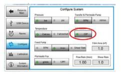
2 The feed pump speed can be altered for CIP if required. Refer section [6.3.1]
