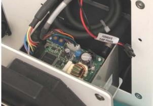
Connect the power cable to the corresponding connection on the permeate pump.
