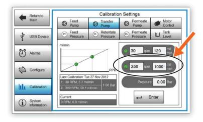
12 The transfer pump is calibrated at 0 bar back pressure.
