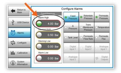
The *Feed Pressure* indicator turns green showing that an alarm high is triggered.
