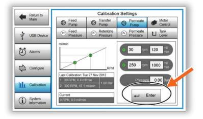
14 To see the flow in ml/min on the main screen after calibration, set the flow rate for the permeate pump to ml/min, see *Set units, on page 167*.
