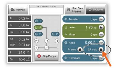
3 To stop the function, tap the *Lock* button and tap *Deactivate* on the displayed keypad.
