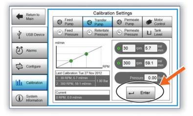
14 To see the flow in ml/min on the main screen after calibration, set the flow rate for the transfer pump to ml/min, see *Set units, on page 167*.
